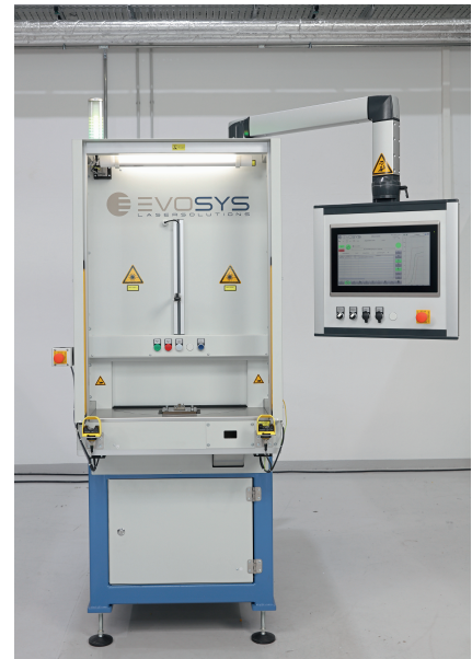
The diode laser of the EVO 1800 joins the parts by contour welding – in twelve seconds per helmet. © Evosys
